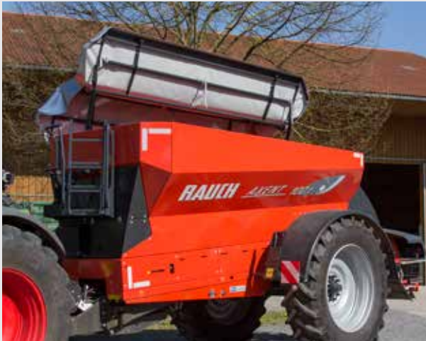
The hopper cover reliably protects the spreading material and can be effortlessly opened
