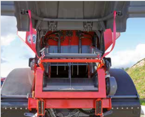
Maintenance flap with gas pressure spring
