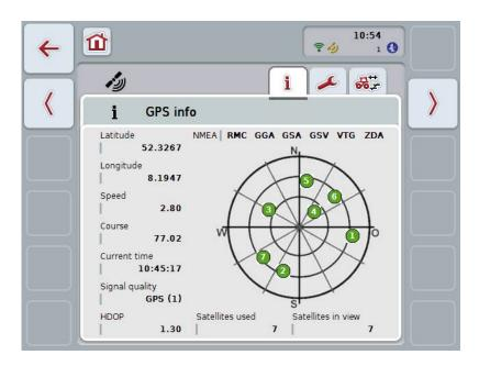
The data are displayed if a GPS receiver is connected, the GPS source and baud rate are correctly selected and the receiver is receiving GPS signals.
