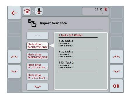
4. Select the task data to be imported. To do so, on the touchscreen press on the button with the task data or change using the buttons "Up" (F10) and "Down" (F11) between the task data or turn the scroll wheel until the button is highlighted in white and press on the "OK" button (F6).
