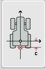
For measuring, marking of the mid-point of the rear axle and the position of the coupling point on the ground using chalk alongside the tractor and then measurement of this distance is recommended.
