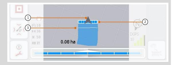
The arrow (1) indicates the position of the tractor reference point (mid-point of the rear axle). According to the set geometries, the sections (2) are positioned behind it. The white line (3) appears if the working depth is set for the sections. This is, for example, supported by a number of fertilizers.
