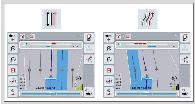
A-B mode: The worker sets an A-point, drives further and sets a B-point. The system automatically draws a line between these two points and in addition creates parallel *guidance tracks* at a distance equal to the working width.
