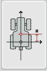
For measuring, marking of the mid-point of the rear axle and the position of the receiver on the ground using chalk alongside the tractor and then measurement of this distance is recommended.
