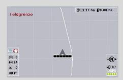
The light grey area is not displayed. The headland is available for working, the sections are not switched off here.
