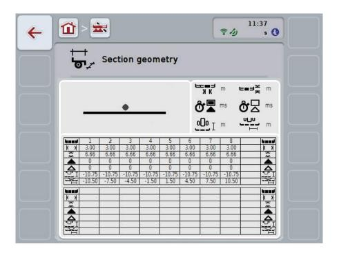
The position of the sections relative to the implement reference point is shown schematically in the top left box. In this way it is possible to see at a glance, whether the sections all lie on a line, or whether different distances have been set in the direction of travel.
