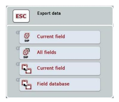
2. Select between "Current field" and "Field database". To do so, press on the button with the desired selection or turn the scroll wheel until the button is highlighted in white and then press on the scroll wheel.
