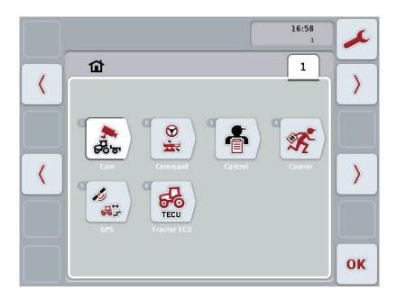
All available apps are shown in the **Main menu**. These are the apps that are enabled on the *terminal*, e.g. CCI.TECU and CCI.Cam and the operating images of the connected implements.
