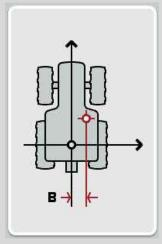
For measuring, marking of the mid-point of the rear axle and the position of the receiver on the ground using chalk to the rear of the tractor and then measurement of this distance is recommended.
