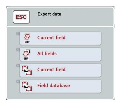
2. Select between "Current field" and "All fields". To do so, press on the button with the desired selection or turn the scroll wheel until the button is highlighted in white and then press on the scroll wheel.
