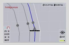
*Guidance tracks* are displayed in the headland. The reference for these *guidance tracks* is the field boundary. The headland can be worked.
