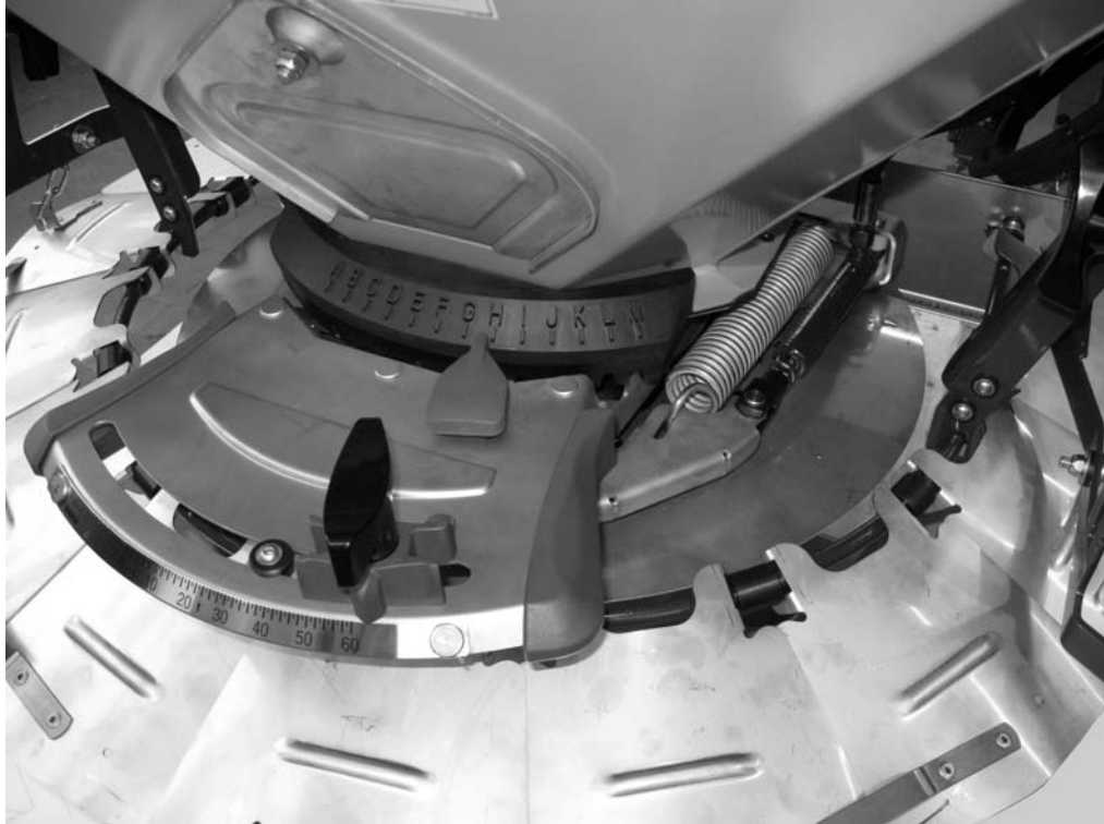
Figure 6.10: Metering slide open, hydraulic cylinder at limit stop
