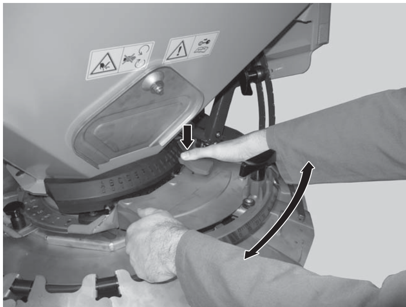
Figure 7.6: Adjustment centre for drop point
