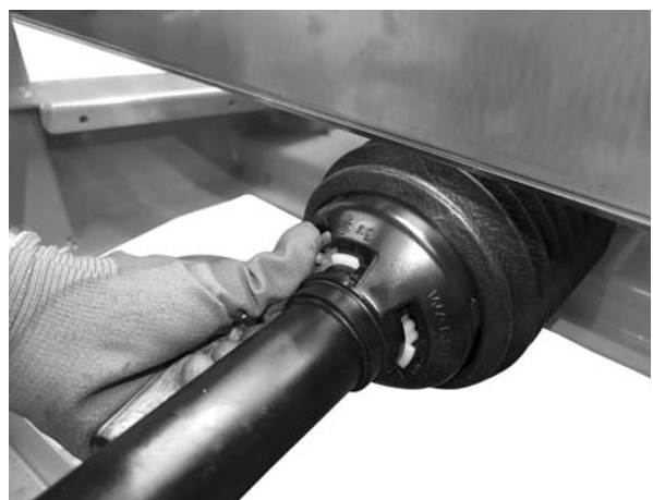
Figure 6.5: Secure the universal drive shaft guard
