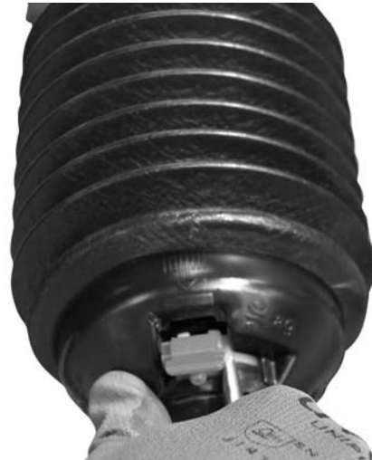
Figure 6.1: Open the universal drive shaft guard
