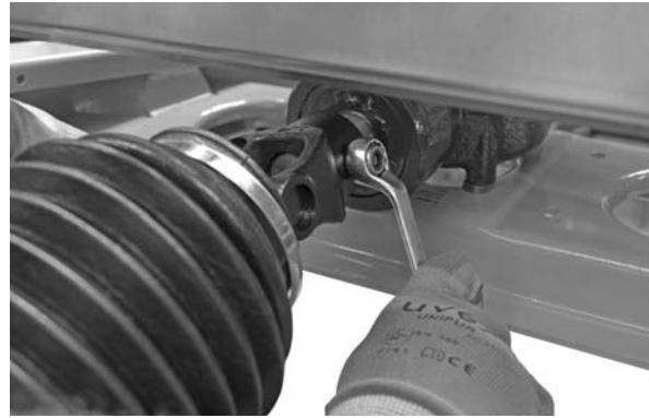
Figure 6.3: Connect the universal drive shaft
