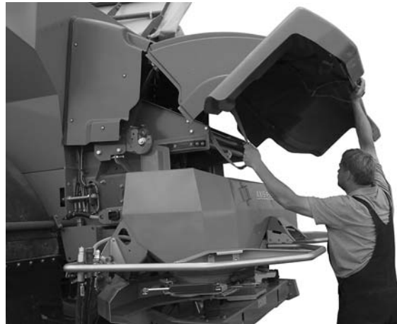
Figure 7.2: Pull the tie cable
