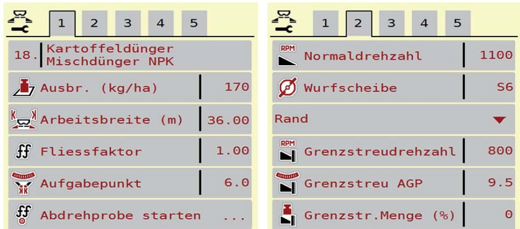
Figure 7.9: Fertiliser settings for full border spreading, AXIS H ISOBUS
