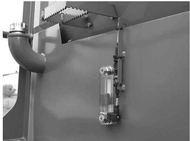
Figure 9.25: Oil filling indicator position
