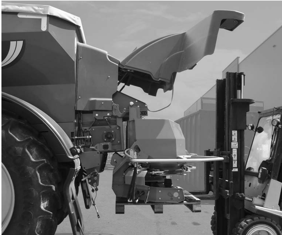
Figure 6.24: Positioning the forklift truck
