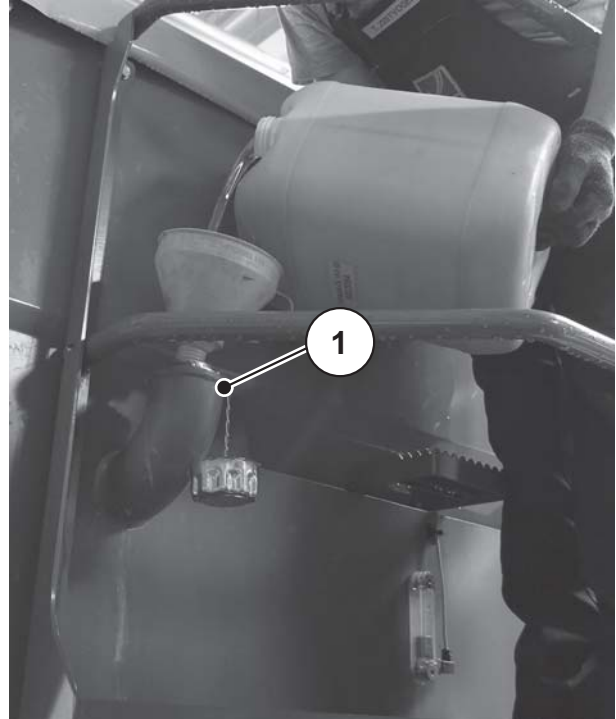
Figure 9.29: Filling in oil
